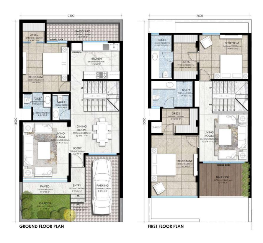
UNIT 02 | PLOT SIZE -24'-6" X 49'-2" (7.5 M X 15M) | PLOT SIZE 1210 sq.ft (112.5 sq.m) BUILTUP AREA 1004.42 sq.ft + 986.17 sq.ft. + 179.30 sq. ft. = 2169.89 sq.ft.
